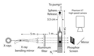
FIG. 2. Schematic of the x-ray setup. The x-ray bending mirror spread the beam and sets the high energy cutoff of 25 keV. The aluminum filter sets the low energy cutoff of 20 keV. The sphere release mechanism consisted of a conical holder with a permanent magnet which held the sphere centered in the holder. A solenoid was used to pull the magnet up and release the sphere.
