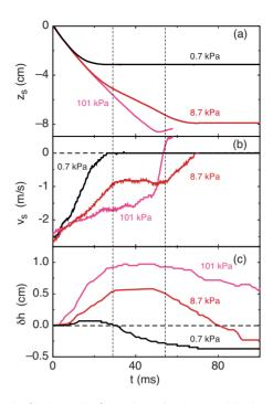
FIG. 13. (Color online) Motion of sphere and bed surface for  $D_s=1.2$  cm. (a) Vertical position  $z_s$  of bottom tip of the sphere as a function of time after impact (at t=0 s). (b) Velocity  $v_s(t)$  computed from curves in (a). (c) Rise of bed top surface.  $D_s=1.2$  cm.
