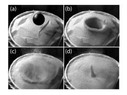
FIG. 9. Scaling up to large grains. Jet formation in  $d \sim 1$  mm corncob pieces at times t=(a)-7.3 ms, (b) 23.3 ms, (c) 173 ms, and (d) 291 ms after impact of a  $D_s=11.4$  cm shot put.
