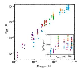
FIG. 6. (Color online) Energy transferred to the jet. Potential energy of the jet at atmospheric pressure is plotted against the kinetic energy of the sphere at impact. Sphere diameter  $D_s = 2.25 \text{ cm}(\mathbf{\nabla})$ , 1.75 cm ( $\mathbf{\Box}$ ), 1.27 cm ( $\mathbf{O}$ ), 0.95 cm ( $\mathbf{\diamond}$ ), 0.79 cm ( $\mathbf{\nabla}$ ), and 0.6 cm (\*). Inset: Ratio of jet potential energy to the spheres kinetic energy at impact vs release height.
