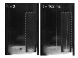
FIG. 4. Effect of boundaries. Jet formation in a 14-cm-diameter container filled 22 cm deep and in a 3.5-cm-diameter container filled 8.5 cm deep (outlined insets). For both cases  $D_s=1.0$  cm,  $H_{drop}=35$  cm, and the bed material was 53  $\mu$ m glass spheres. The images for the big and small container have the same horizontal and vertical scales, and the insets are shifted such that the impact points of the sphere and the bases of the two jets line up.
