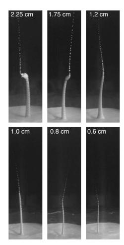
FIG. 7. Changing the sphere diameter. Images of the jet at its maximum height for  $P_0=13.3$  kPa and  $H_{drop}=1.1$  m varying  $D_s$  from 2.25 to 0.6 cm.
